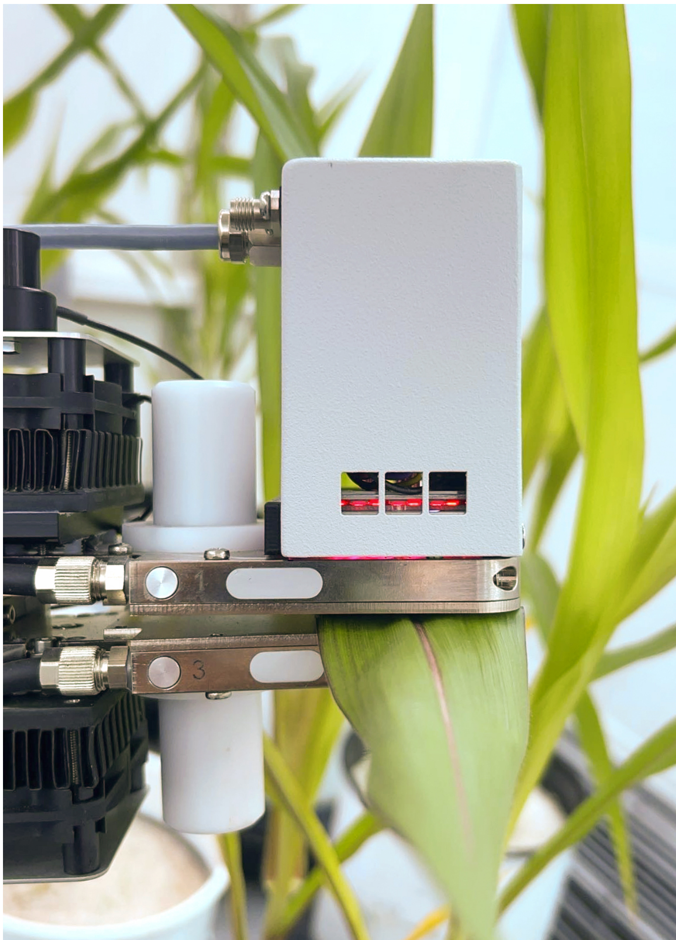
Measuring gas exchange parameters with a GFS (Walz) after application of leaf fertilizer on maize plants. (Photo: Lass)
