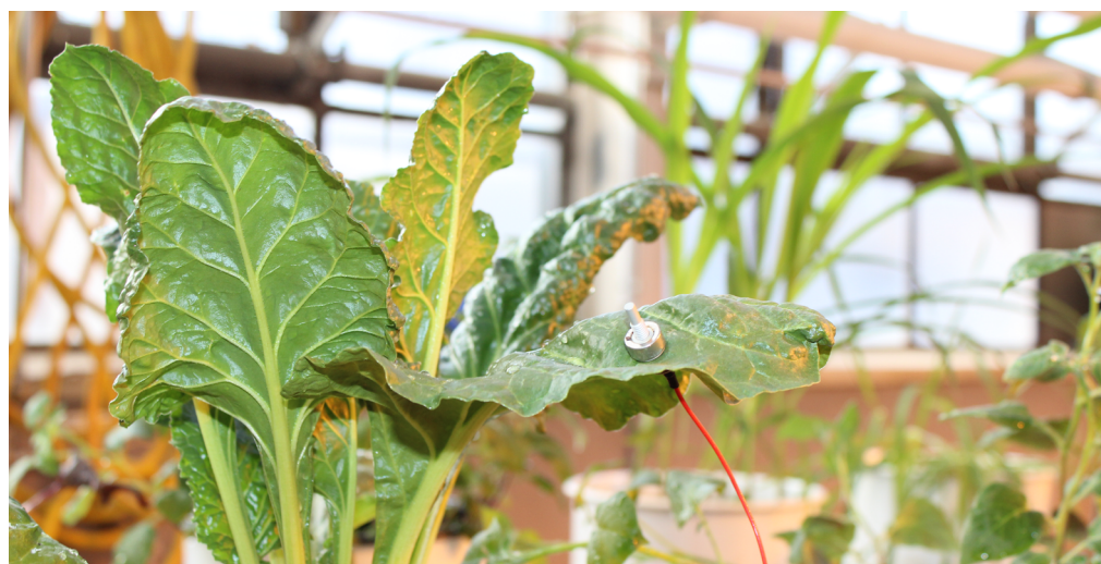
A leaf patch clamp pressure (LPCP) probe applied on a leaf of a sugar beet plant. (Photo: Cabrita)
